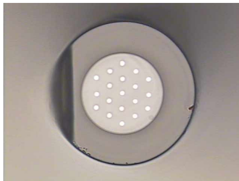
Fig. 1. Cross-section of the image amplifying fiber.
